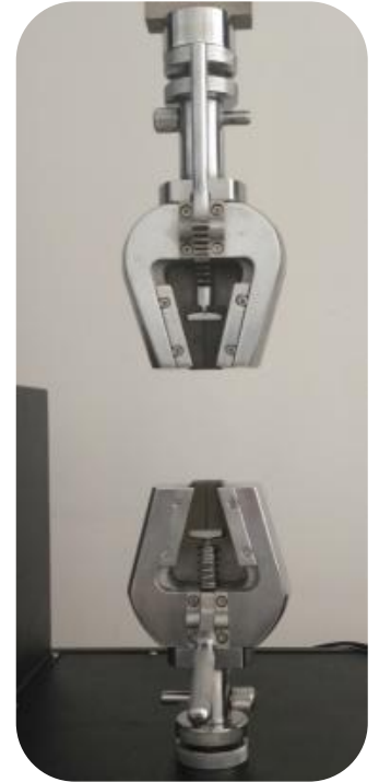
Tensile clamp Material:stainless steel Open mouth:0-10mm
